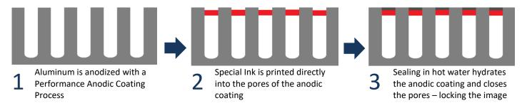
Conventional Printing - Steriscreen Anodize with Epoxy Ink Print
